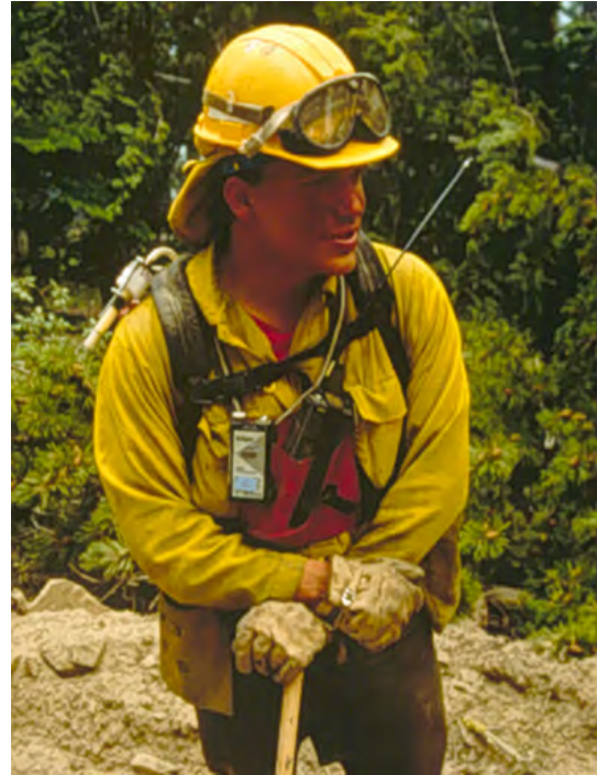
Figure 2.2.3. Backpack sampler capturing particulate matter, acrolein, formaldehyde, and other smoke exposure compounds within several inches of a workers face. Note the electronic dosimeter for testing.
