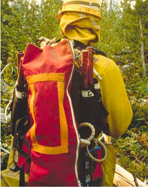
Figure 2.2.2. Backpack sampler and pumps worn by firefighters to capture smoke exposure samples.
