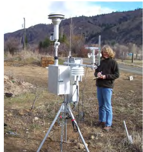
Figure 5.4.4. Beta attenuation monitors, like the rugged and portable E-BAM, are accurate and well-suited for smoke monitoring applications.
