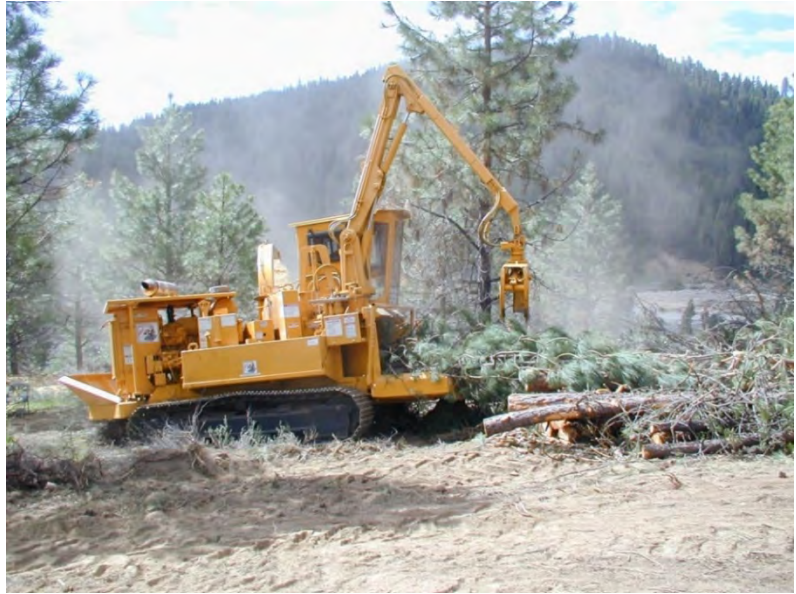
Figure 4.2.2. Mechanical processing of biomass.
