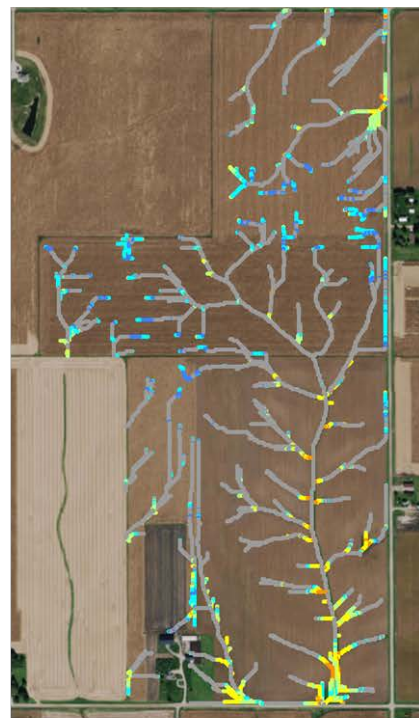
EphGEE deposition in gully channels
