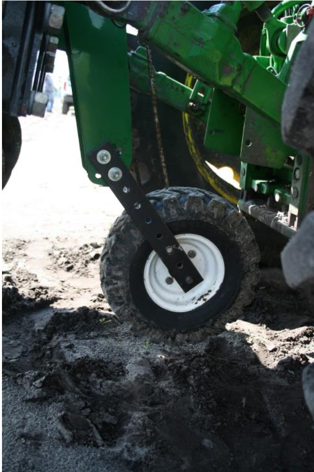
Great Plains 3P605 NT Drill with raised drive wheels
